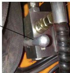
Driewegklep in horizontale positie (ON)
