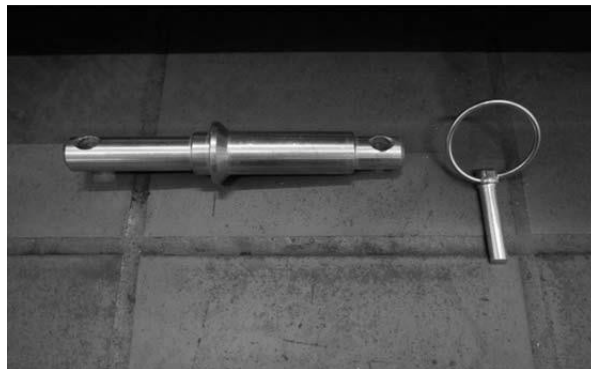
Fig. 39 Reversible bolt with retaining pin
