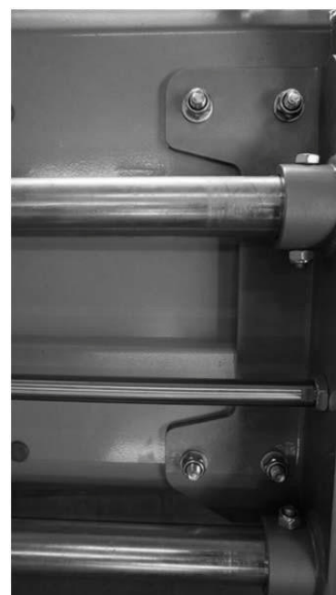
Fig. 15 Mounted hydraulic lateral shifter (right side)
