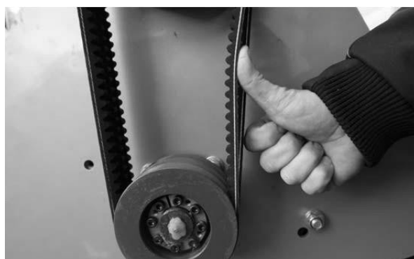
Fig. 26 Correct drive belt tension
