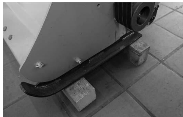
Fig. 10 Jacking up the mulcher
