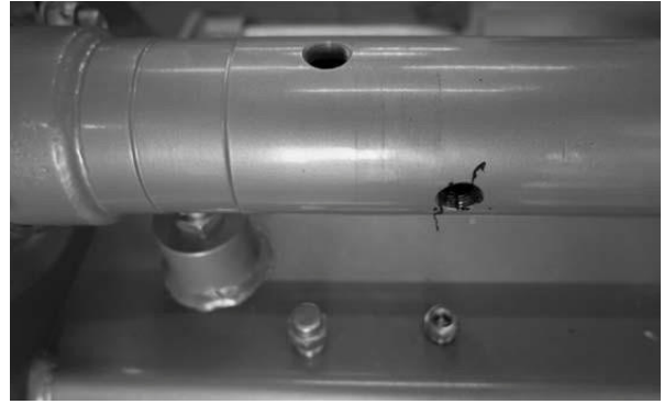
Fig. 30 Drive shaft with inspection port and filling port
