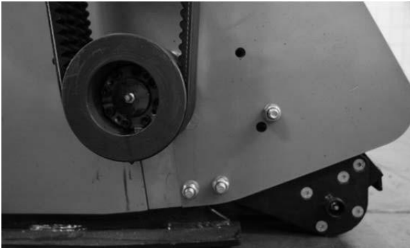
Fig. 31 Smeernippel in rijrichting, links
