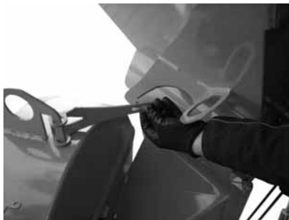
Locking the feed hopper
