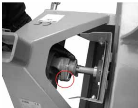
Assemble the power take-off
