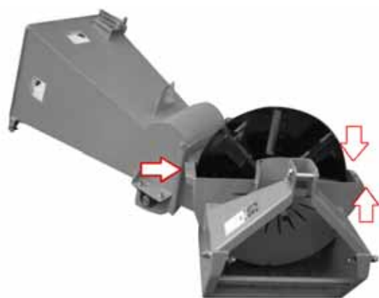
Loosen the screws
