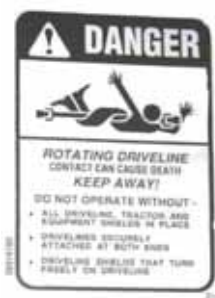
A danger decal on the protection of the power take-off shaft.
