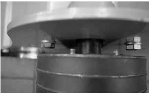
Fig. 25 Correct drive shaft distance
