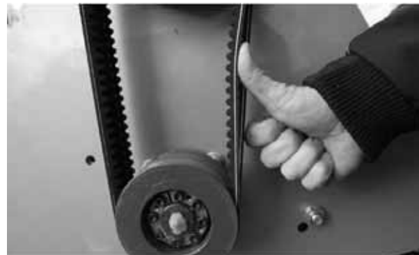
Fig. 26 Correct drive belt tension
