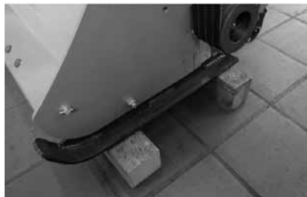
Fig. 10 Jacking up the mulcher
