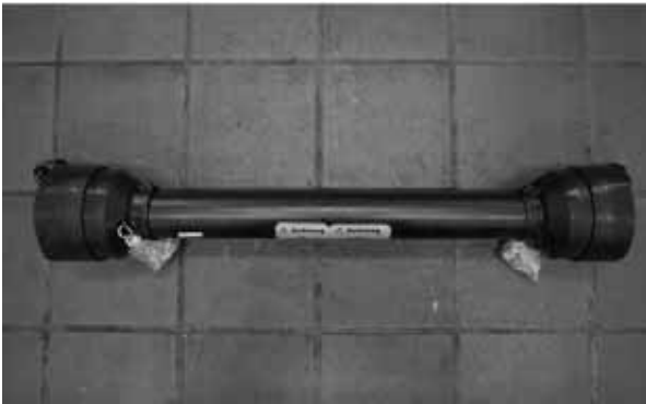
Fig.41 Power take-off with guard and chains
