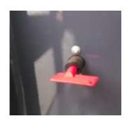
The lever can be removed when switched off. This provides additional protection from theft.
