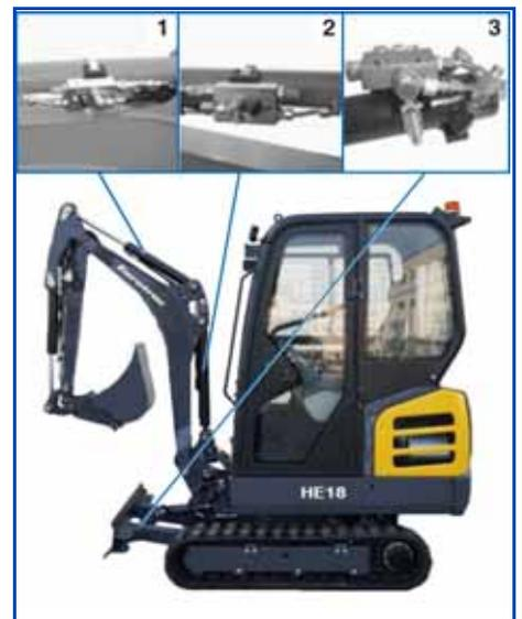
If the dozer blade is used for support, an additional line rupture protection must be installed in accordance with EN 474-1 to increase the stability of the machine.
